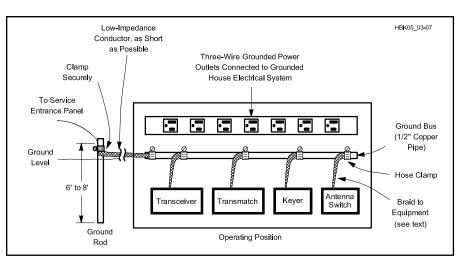
Fig 28.5 — An effective station ground bonds the chassis of all equipment together with low-impedance conductors and ties into a good earth ground. Note that the ground bus is in turn bonded to the service entrance panel. This connection should be made by a licensed electrician with #6 AWG (minimum size) copper wire.
