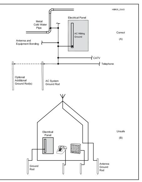
Fig 28.6 — At A, proper bonding of all grounds to electrical service panel. The installation shown at B is unsafe — the separate grounds are not bonded. This could result in a serious accident or electrical fire.
