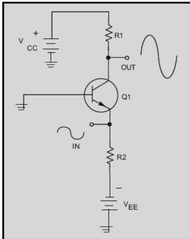
Figure 1-4 A simple class A transistor amplifier
