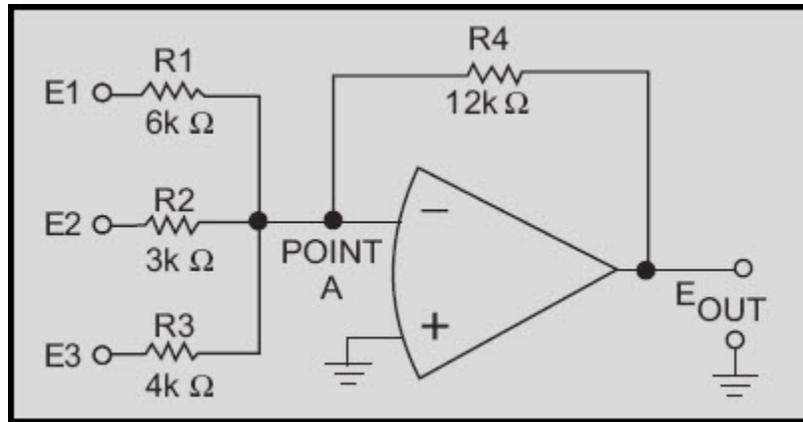
Figure 3-24 Scaling amplifier
