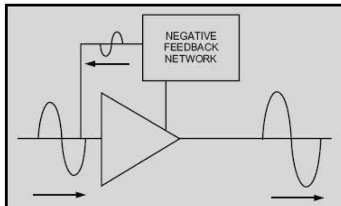
**Figure 1-17D.—Feedback uses in amplifiers**
