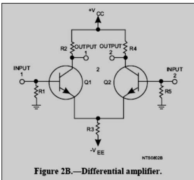
IN ANSWERING QUESTIONS 2-11 THROUGH 2-24, REFER TO FIGURE 2B AND THE FOLLOWING INFORMATION: ALL INPUT SIGNALS ARE SINE WAVES WITH A PEAK-TO-PEAK AMPLITUDE OF 5 MILLIVOLTS. THE GAIN OF THE AMPLIFIER IS 100.
