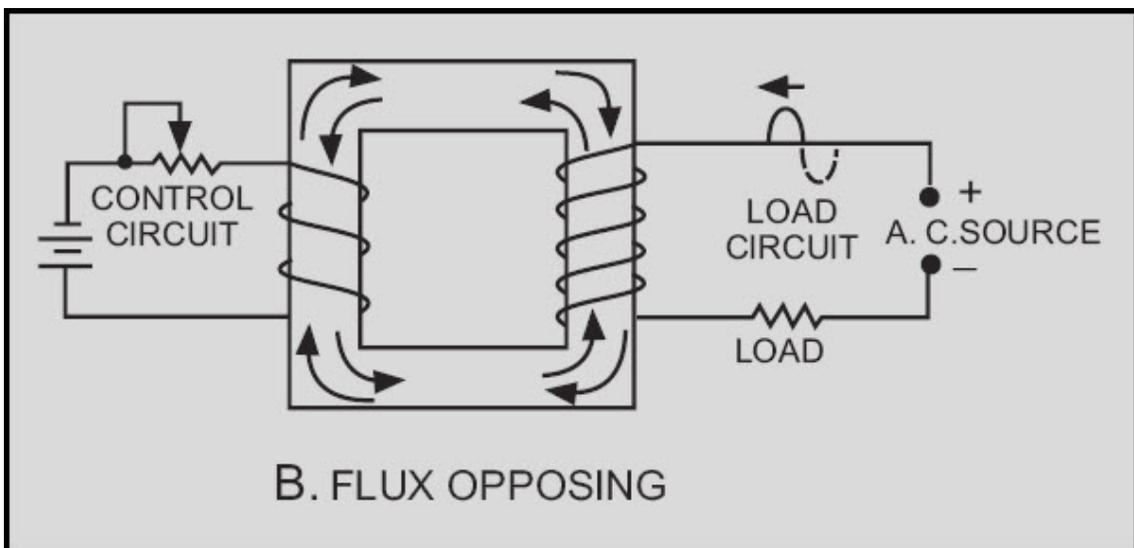
**Figure 3-35B.—Flux paths in a saturable-core reactor. FLUX OPPOSING**
