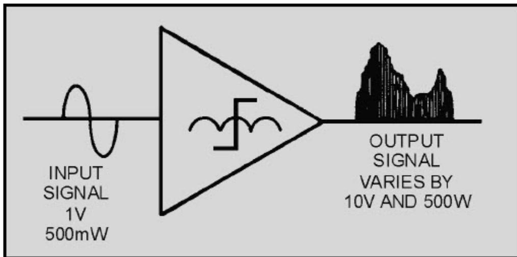
Figure 3-41 Magnetic amplifier input and output signals
