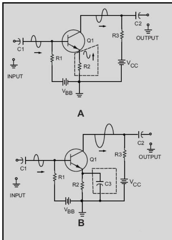
Figure 1-20A-B Decoupling (bypass) capacitor in a transistor amplifier
