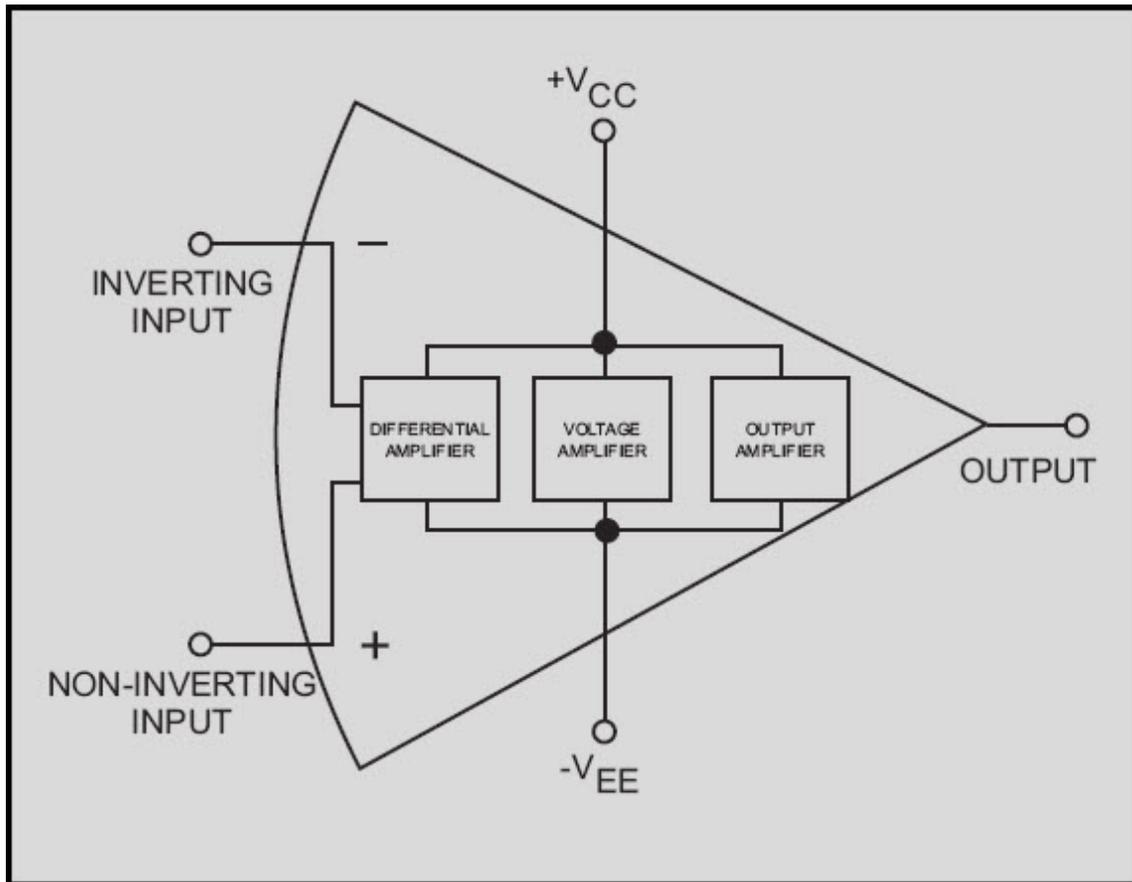
**Figure 3-11 Block diagram of an operational amplifier**
