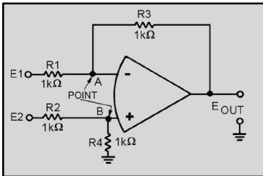
Figure 3-25 Subtractor circuit
