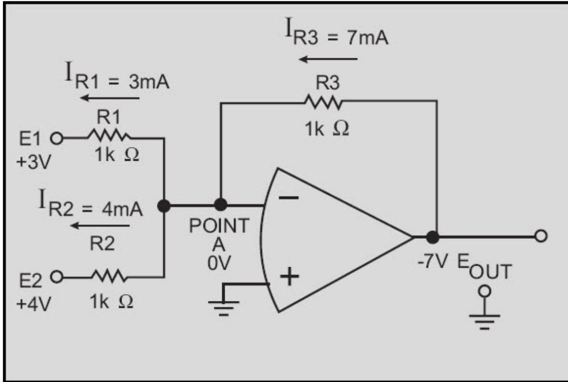
Figure 3-21 Current and voltage in a two-input adder
