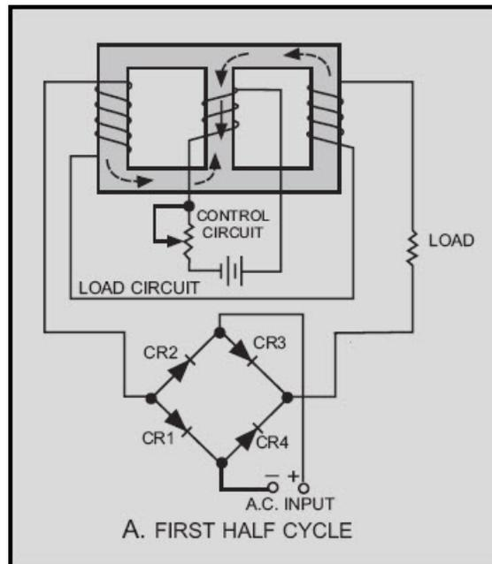
Figure 3-39A Simple full-wave magnetic amplifier. FIRST HALF CYCLE
