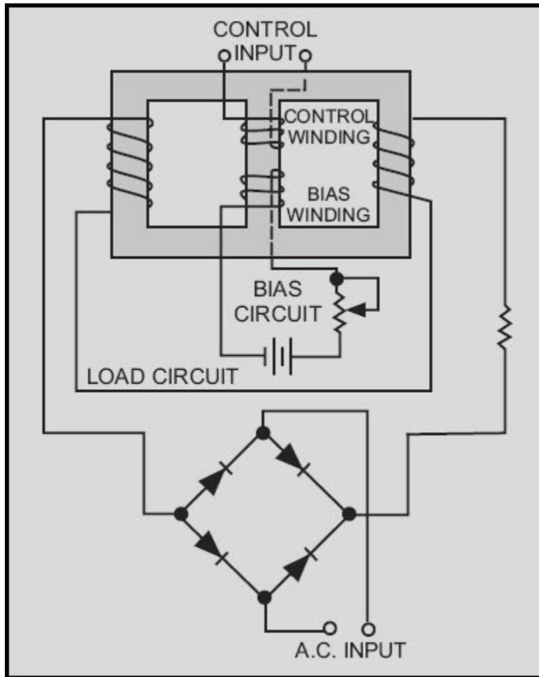
Figure 3-40 Full-wave magnetic amplifier with bias winding
