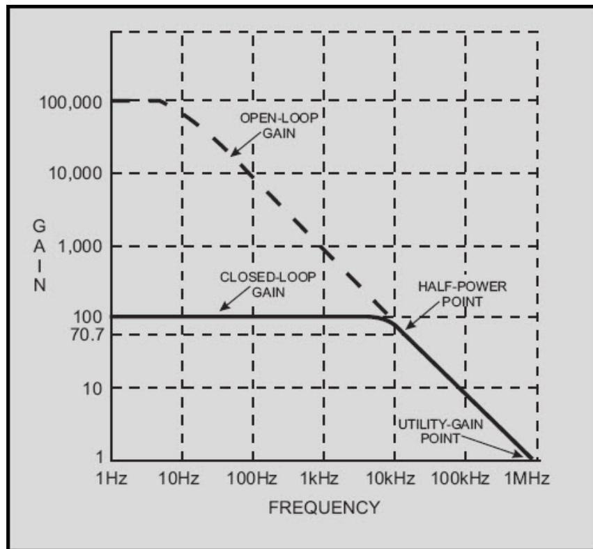
Figure 3-18 Closed-loop frequency-response curve for gain of 100
