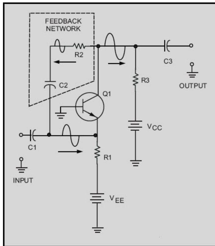
Figure 1-18 Positive feedback in a transistor amplifier
