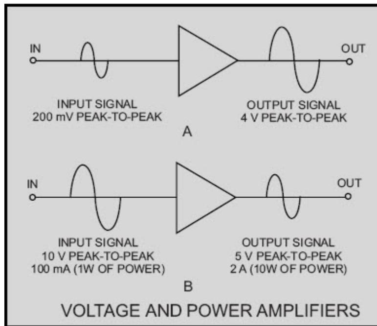
**Figure 1-3 Diagram of voltage and power amplifiers**
