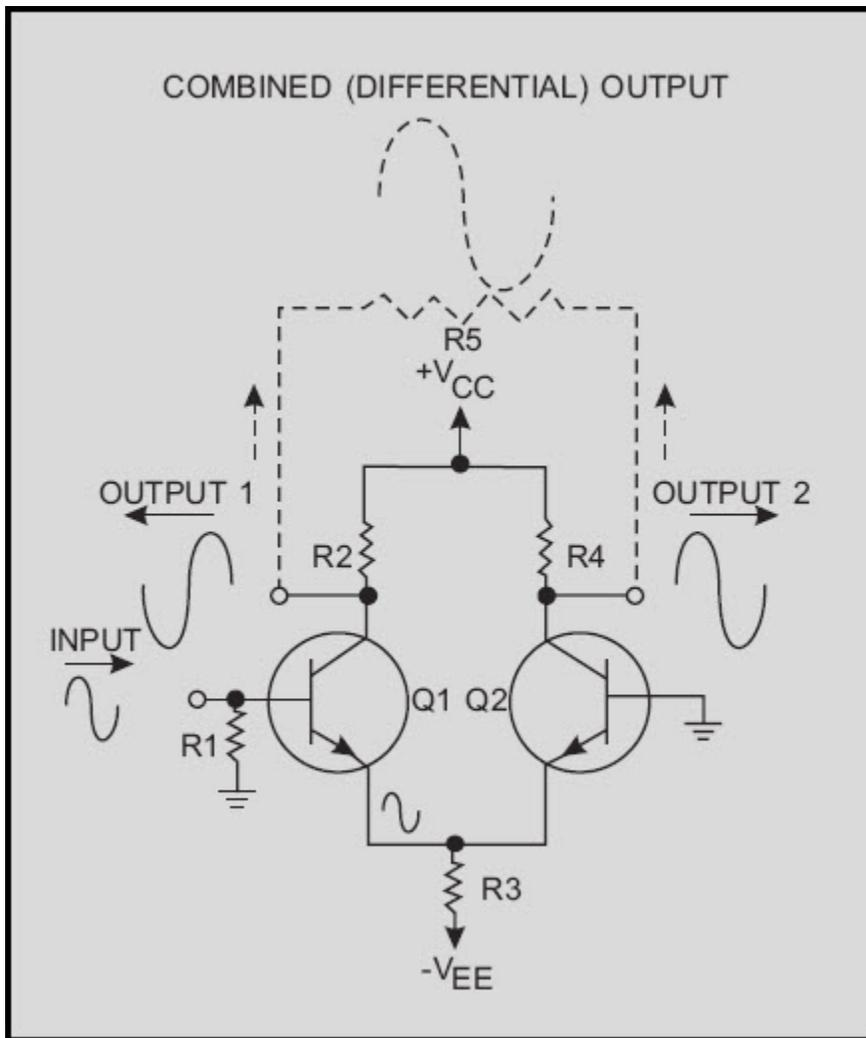
Figure 3-8 Single-input, differential-output differential amplifier
