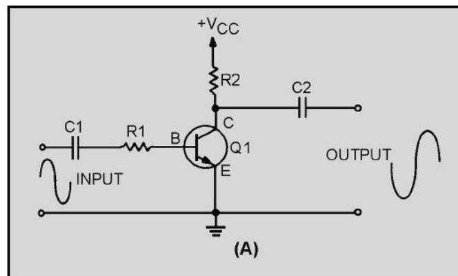
Figure 3-1A Common-emitter and common-base amplifiers
