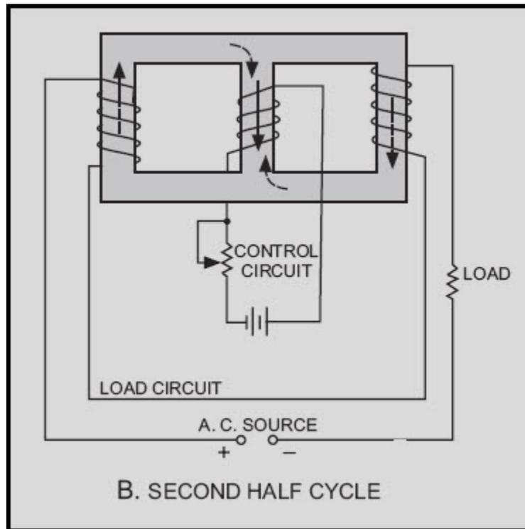
**Figure 3-36B.—Three-legged, saturable-core reactor.
