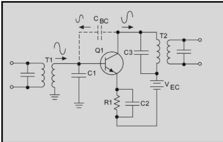
**Figure 2-17 Interelectrode capacitance in an rf amplifier**
