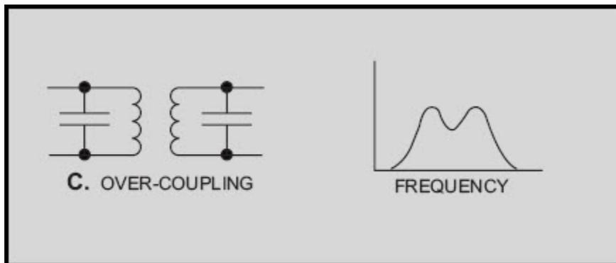
**Figure 2-16C.—Effect of coupling on frequency response. OVER-COUPLING**
