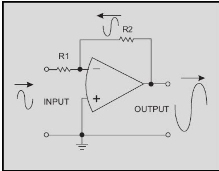
**Figure 3-13 Inverting configuration**
