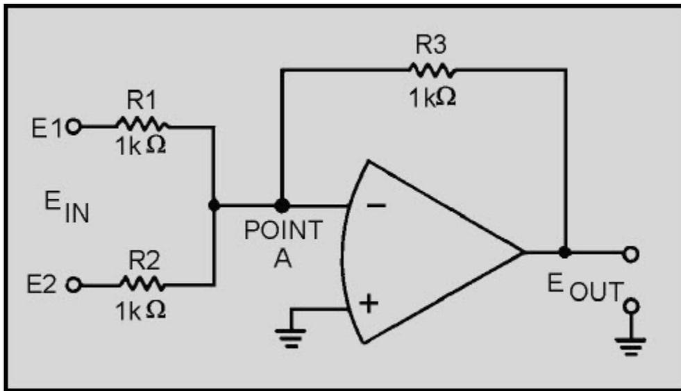
**Figure 3-20 Two-input adder**
