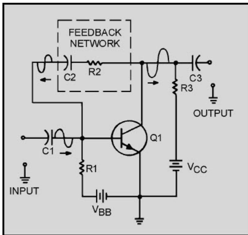
Figure 1-21 Negative feedback in a transistor amplifier
