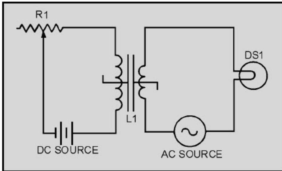
Figure 3-33 Schematic diagram of a simple saturable-core reactor
