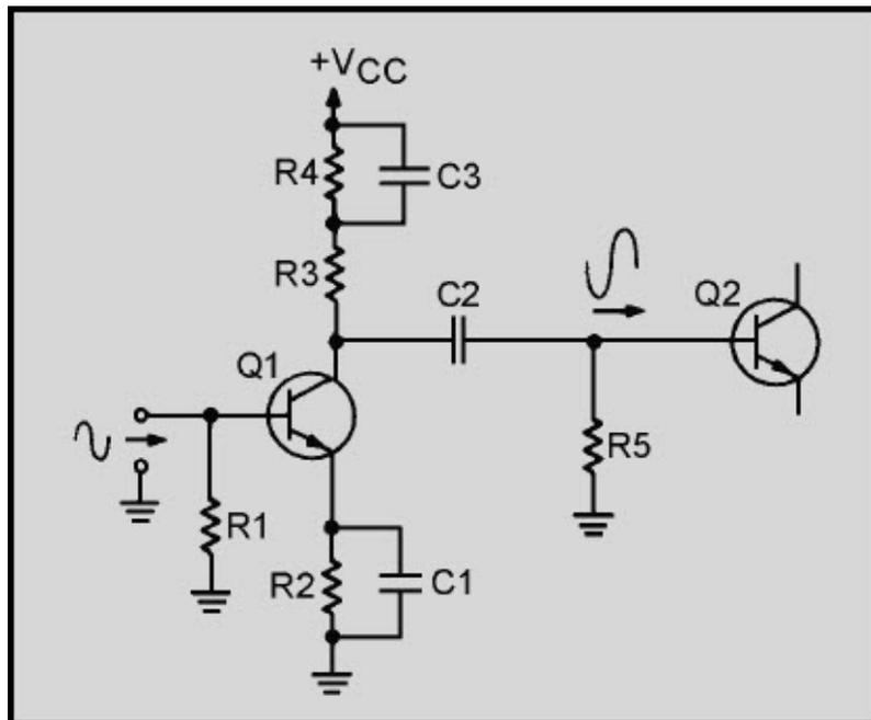
Figure 2-9 Low frequency compensation network
