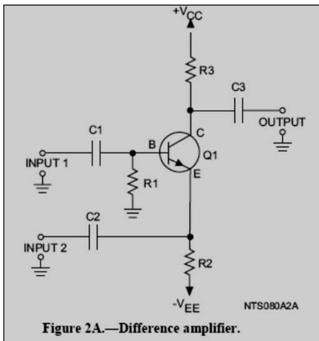
IN ANSWERING QUESTIONS 2-3 THROUGH 2-10, REFER TO FIGURE 2A AND THE FOLLOWING INFORMATION: THE AMPLIFIER HAS A GAIN OF 6 AND THE INPUT SIGNALS ARE SINE WAVES WHICH ARE EQUAL IN AMPLITUDE AND VARY BETWEEN +2 VOLTS AND -2 VOLTS.
