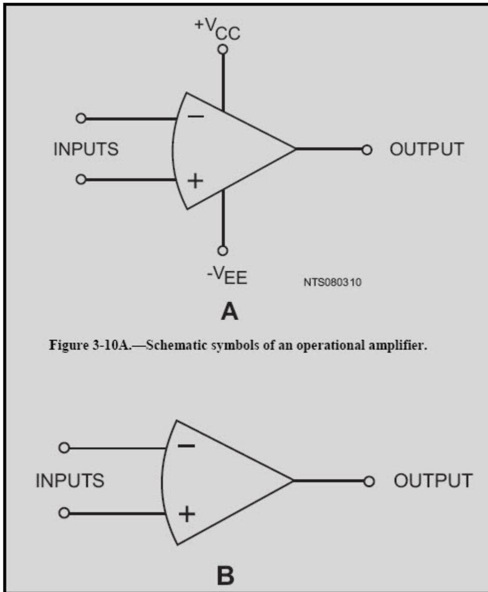
Figure 3-10A.—Schematic symbols of an operational amplifier.
