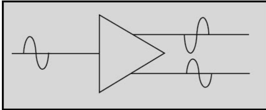
Figure 1-26 Block diagram of a phase splitter
