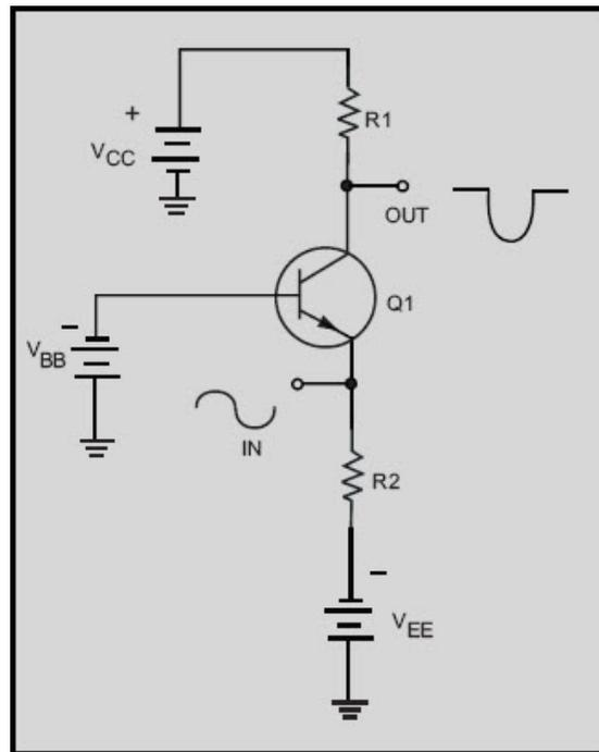
Figure 1-7 A simple class C transistor amplifier
