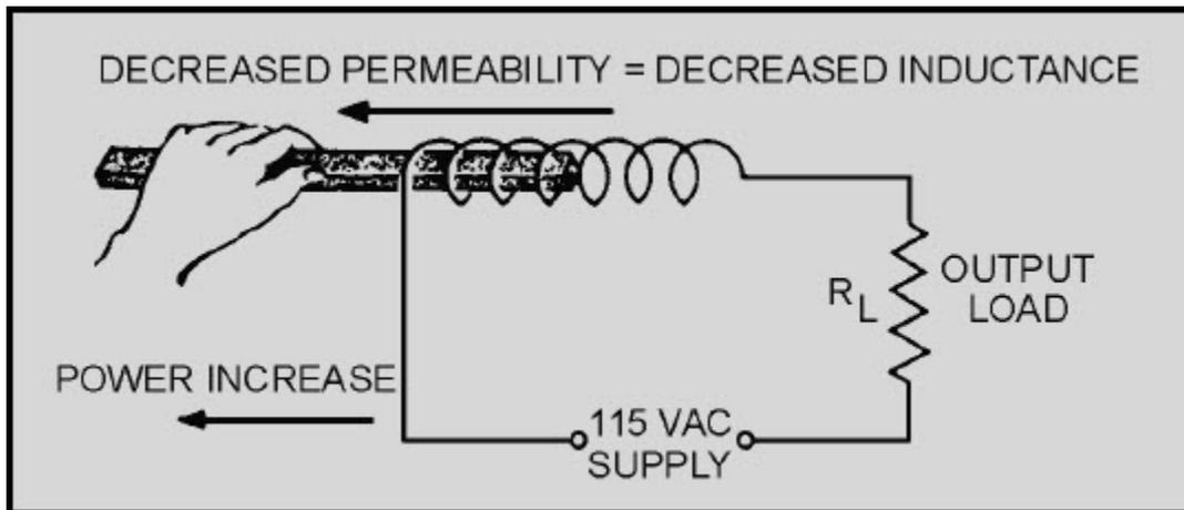
Figure 3-30 Varying coil inductance with a movable coil
