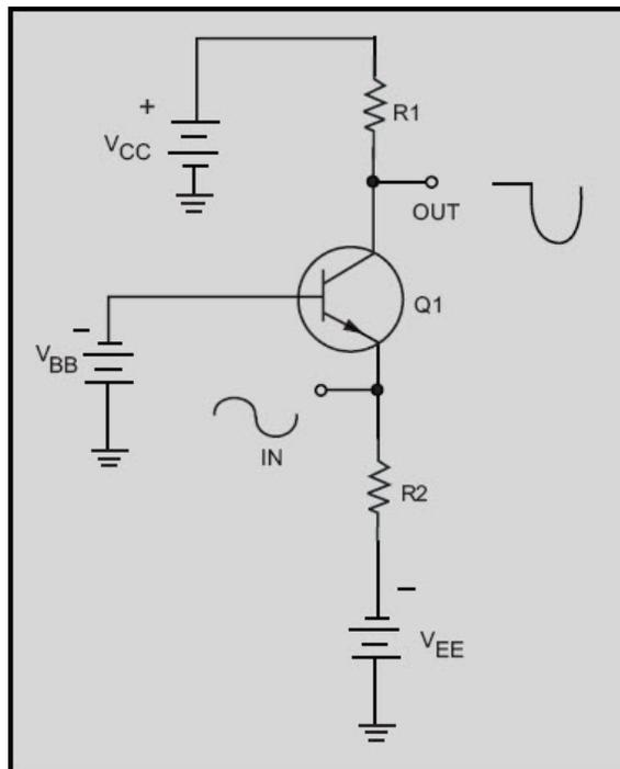
Figure 1-6 A simple class B transistor amplifier
