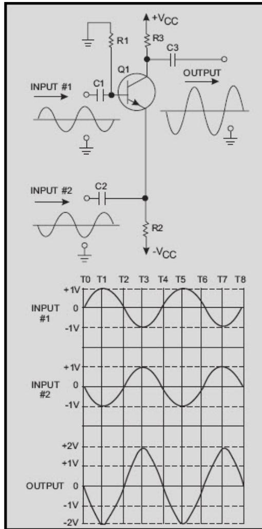
Figure 3-3 Input signals 180° out of phase
