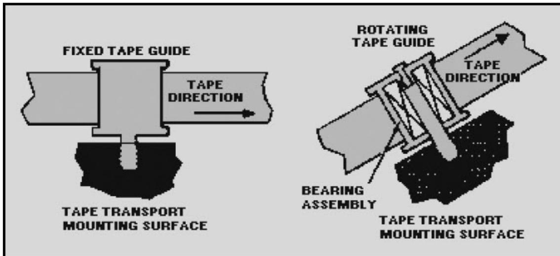
Figure 4-6 Typical fixed and rotary tape guides
