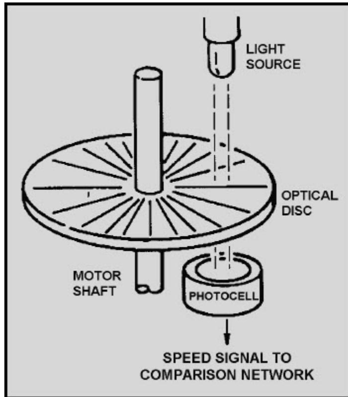
Figure 4-15 Capstan speed monitor using a photo-optical tachometer
