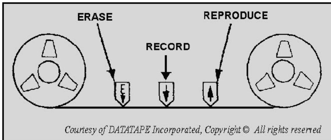
Figure 3-3 Placement of magnetic tape recorder heads
