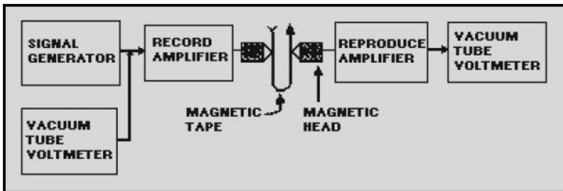
Figure 6-1 Test equipment setup for measuring signal-to-noise ratio
