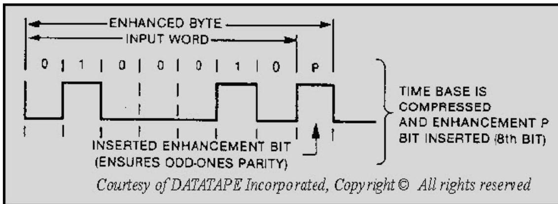
Figure 7-5 Enhanced non-return-to-zero-level (E-NRZ-L) digital encoding method
