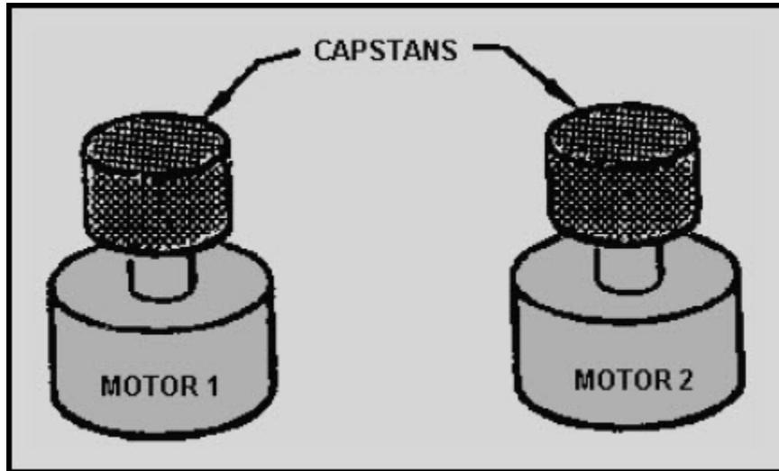
**Figure 4-12 Dual-motors dual capstans drive system**
